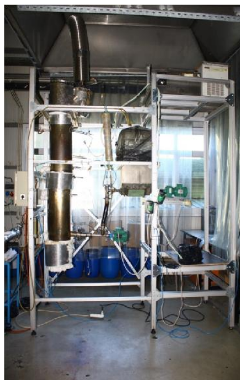
10 kWth Biomass Gasification
